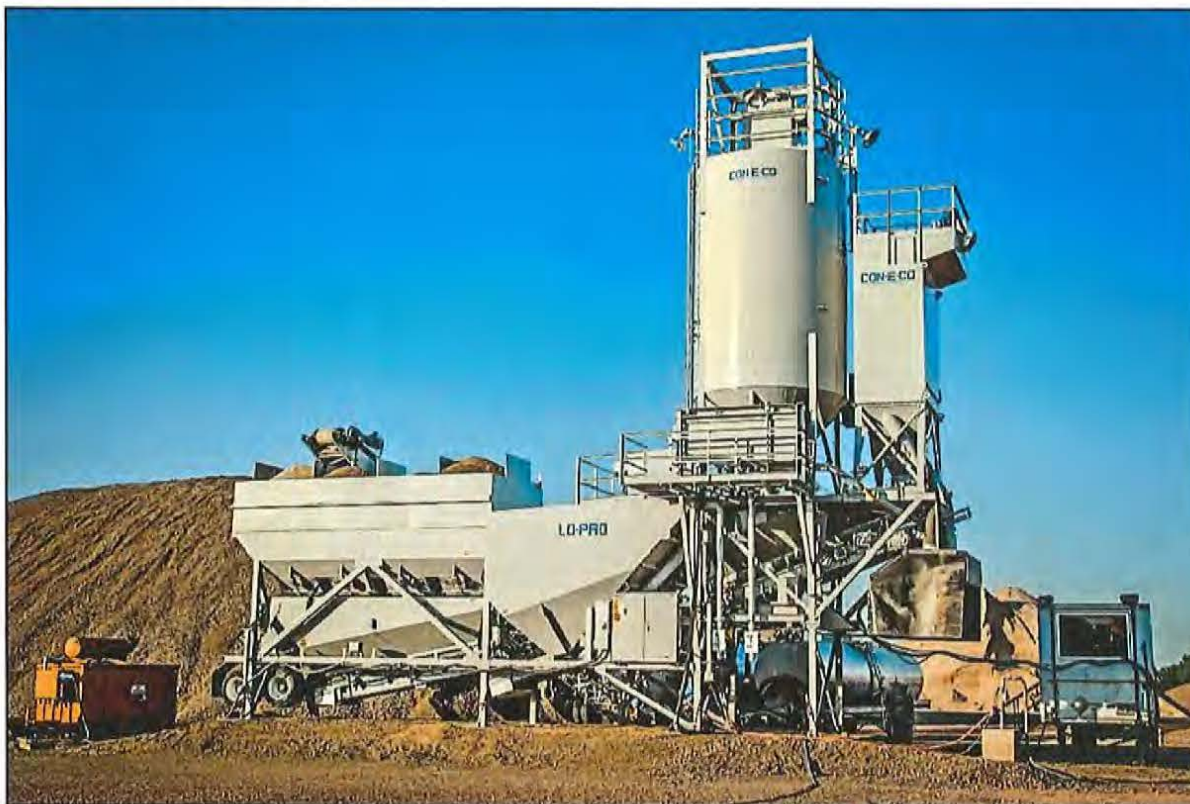
Figure 4 – Concrete Batch Plan (Typical) 2
