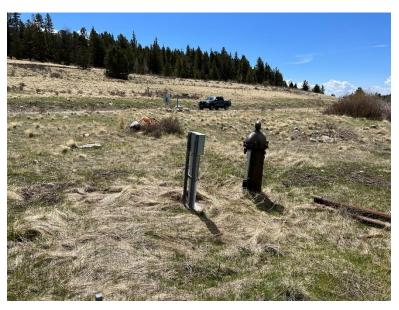
Well #4 is located between Well #3R and Well #2R along the west edge of the gravel access road east of the pond on the WTP property. The well is the original well, constructed in 1989. A Well #4R was redrilled in 2007 near the existing well but did not produce sufficient water and was permitted as a monitoring well. Well #4 has a completed depth of 47-feet. The well is permitted for 300 gpm and includes a submersible pump
